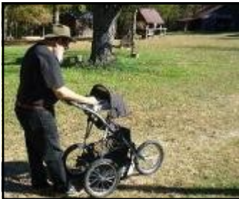
Dan Elliot using the GPR to survey the side yard of Fort Hollingsworth
